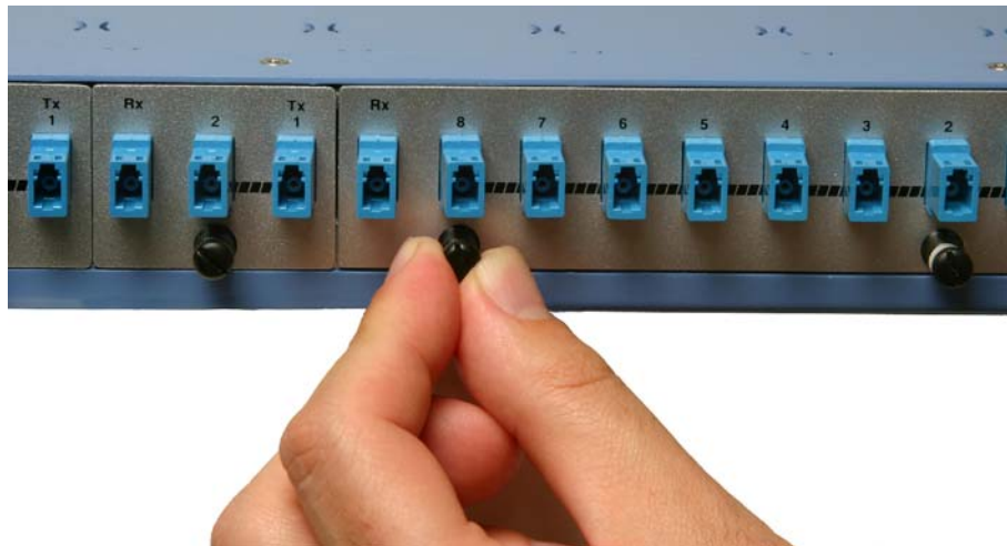
Figure 2-2 Unscrewing Captive Screw
