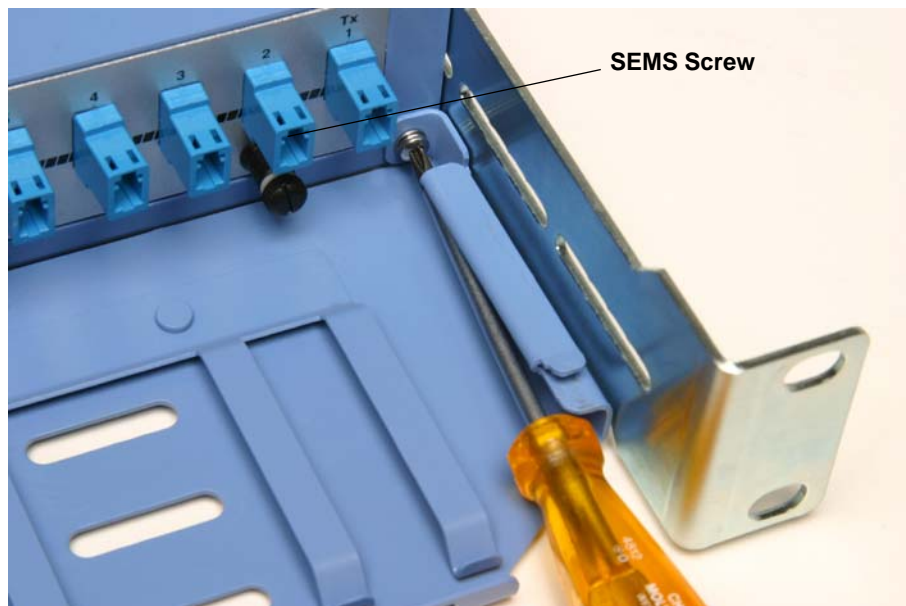
Figure 2-10 Removing the Vertical Edge Tongues of the Cable Management Shelf
