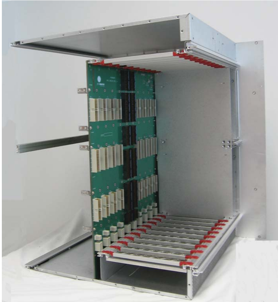
Figure 2-10 Chassis after Removal of Left Side Panel
