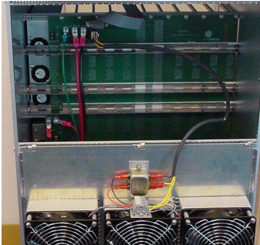
Figure 2-3 Rear Panel with Fan Assembly Door Hanging Freely
