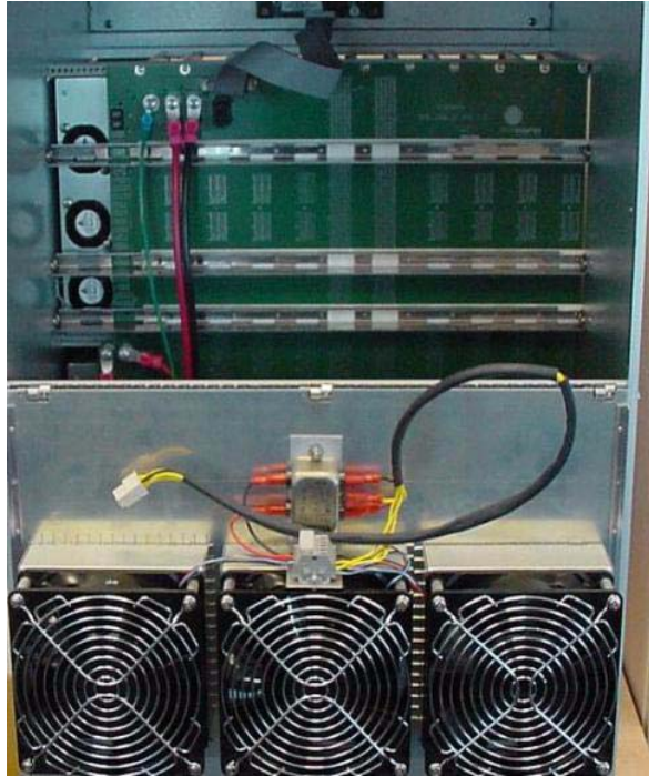
Figure 2-5 Removing the Fan Cable from the Chassis Interior
