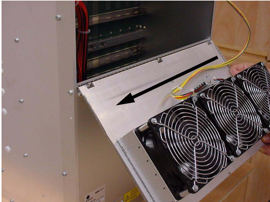
Figure 2-6 Rear Panel Fan Assembly Removal
