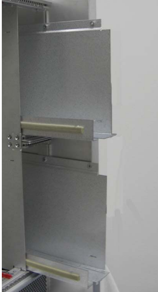
Figure 2-16 Removing the Power Supply Shelves
