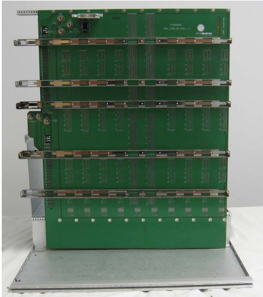
Figure 2-17 Chassis Rear View - after Removing Top and Side Covers
