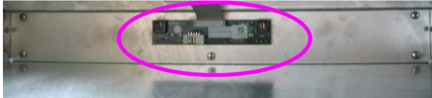
Figure 2-13 Removing the LED Card from the Top Cover (Top Cover Upside Down, view from Back)
